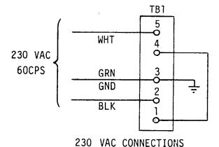
Termination of AC Power Cord at Terminal Strip TB1
